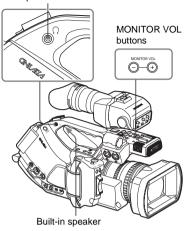
With the headphones connected to the headphone jack, the built-in speaker is turned off.
